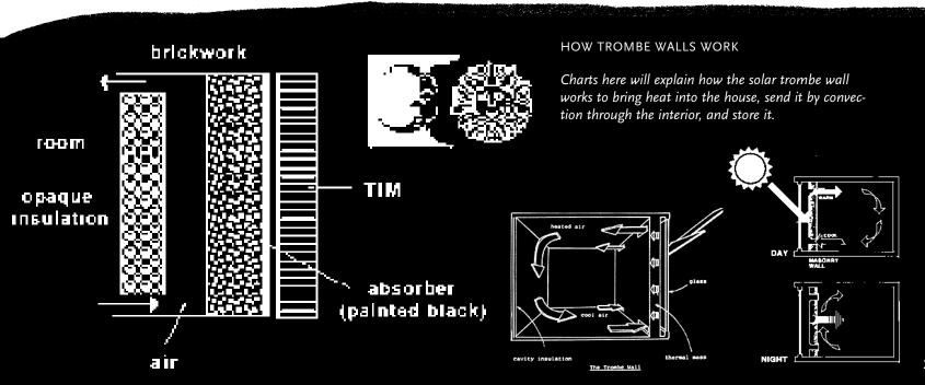
While the fancy view and custom details make Hill House feel like a luxury dwelling, many features of the house show its earthy roots. The only heat source in the house besides the handmade woodstove is a passive solar trombe wall, designed to feed warm air into the house or vent it out by natural convection. A traditional farm windmill pumps water from the well, which is deliverd to the house via gravity feed and heated with solar panels.
